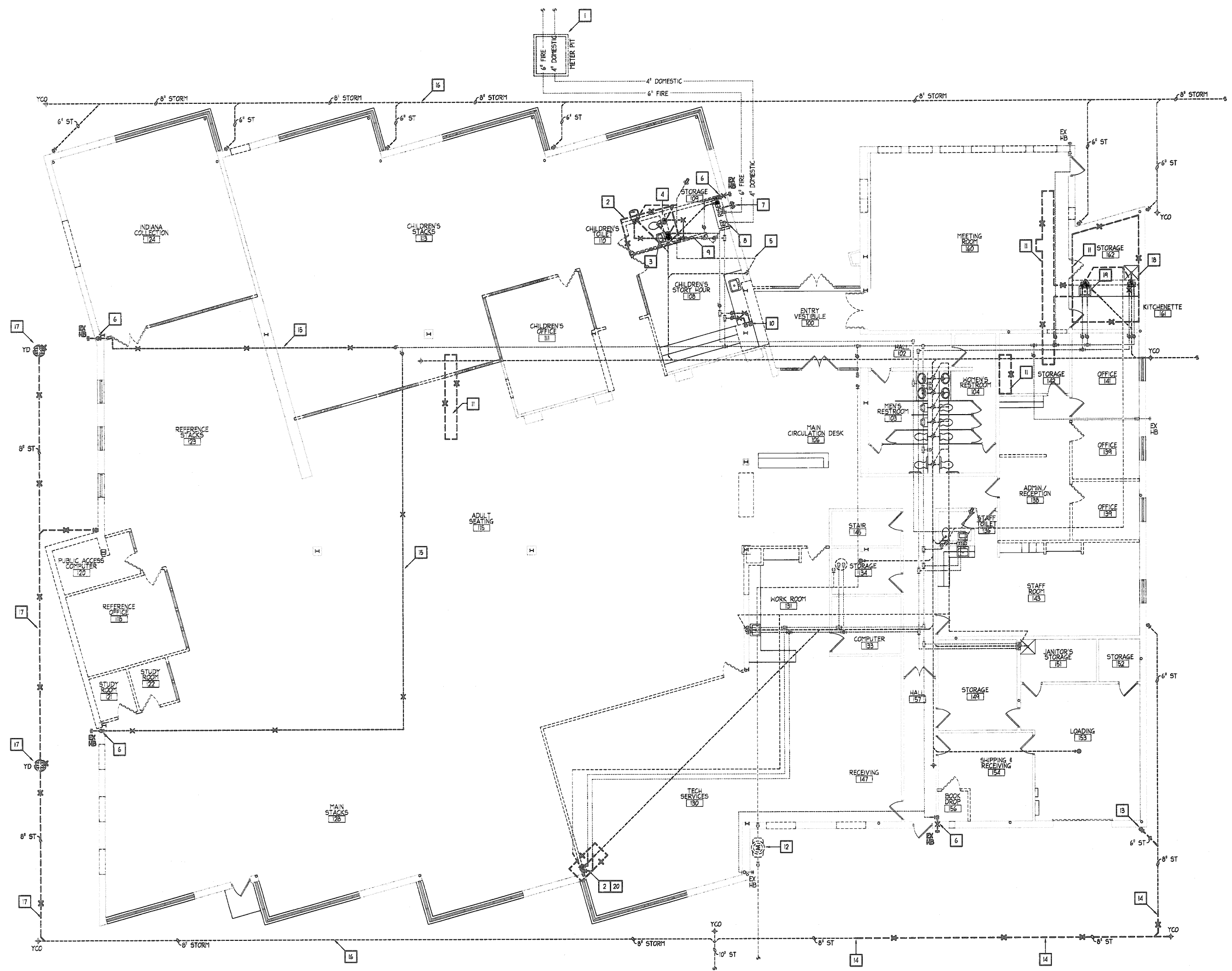
PLUMBING DEMOLITION PLAN SCALE: 1/8" = 1'-0" NORTH
